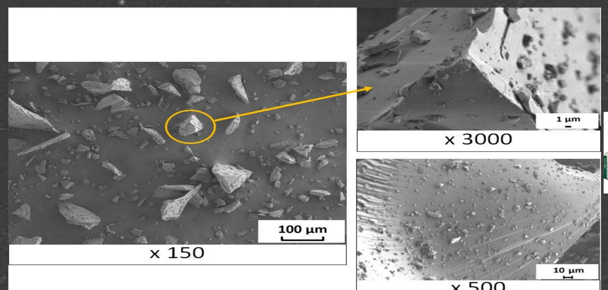
Image 3. Micrographs of borpolymer particles
