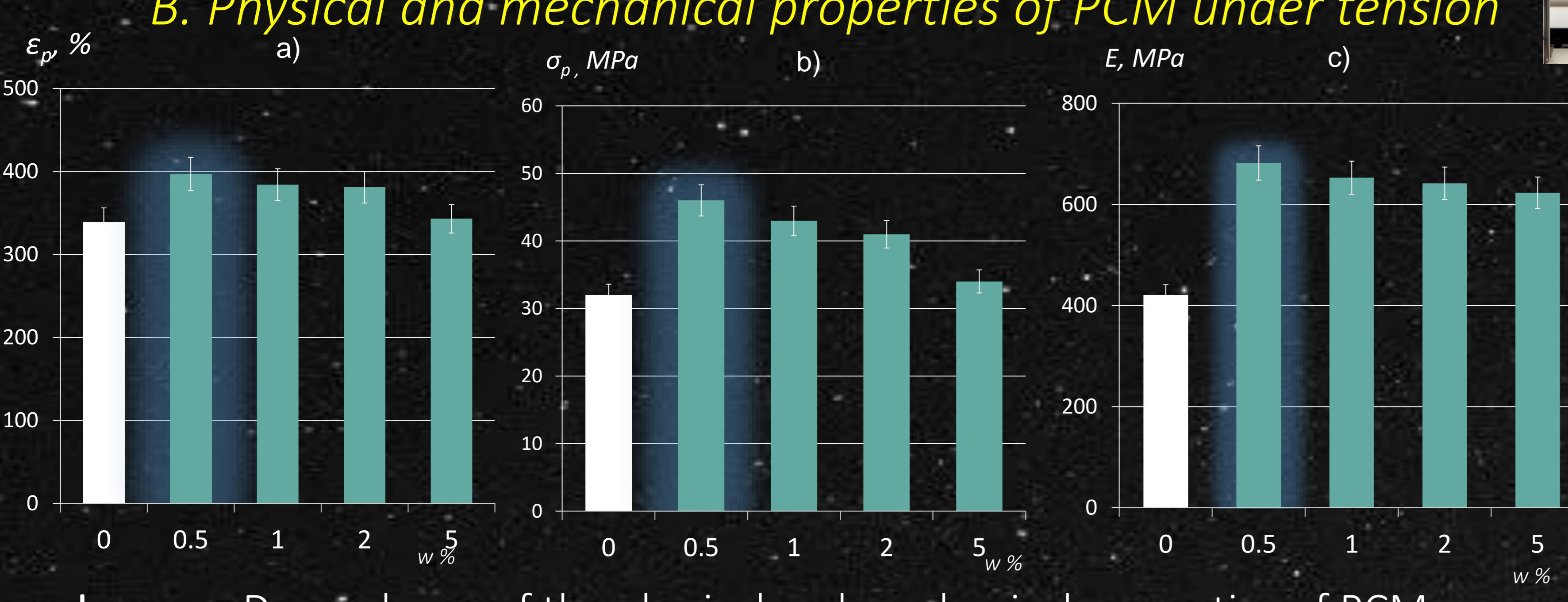
Image x. Dependence of the physical and mechanical properties of PCM on the borpolymer content:: a)  $\varepsilon_p$  – elongation at break, %; b)  $\sigma_p$  – tensile strength, MPa; c)  $E_p$  – modulus of elasticity, MPa.
