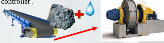
Input parameters: - supply of ore to the mill, **QP**, t/h; - water consumption in the mill, **QB**, m<sup>3</sup>/h;
